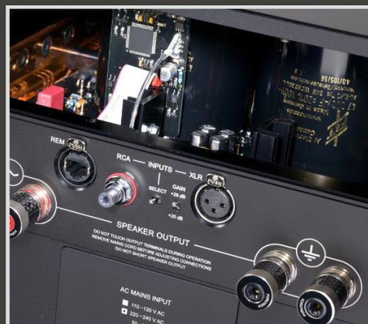
... except flexible wires to the huge suspended toroid, there is not even one signal or supply cable.
