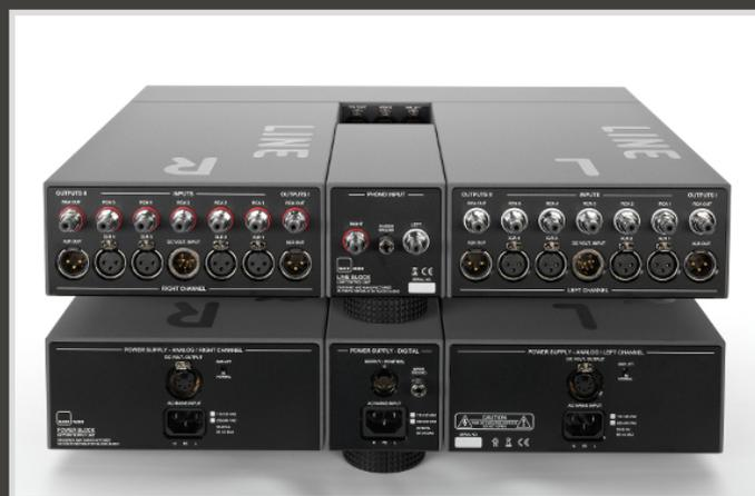
... the Line & Power construction is divided into seven physically separated, shielded and electrically isolated cases.
