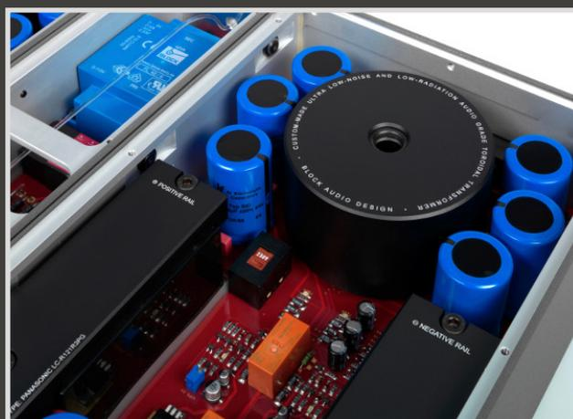
... volume control and inputs switching are provided by precision (Mu-Metal shielded) reed relays from Pickering. Toroidal transformer in the Power Block is actually hanging on a single silent-block!
